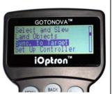
**Step 16. Sync to Target** (Use this to center and synchronize the object selected in Step 15).
