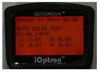
Now the kit motors can be controlled by a guiding signal from an ST-4 compatible autoguiding equipment through Guide Port. Use the number key to select guide rate.
