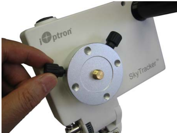
Figure 15. Remove camera mounting block
