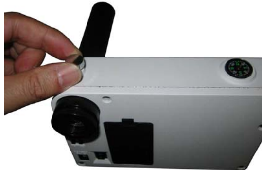
Figure 12. Installed polar scope
