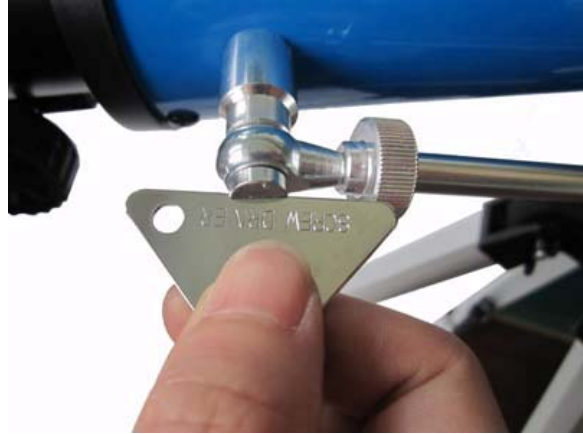
Figure 6. Install Altitude adjustment rod
