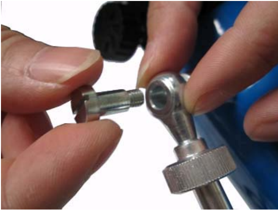
Figure 6. Install Altitude adjustment rod
